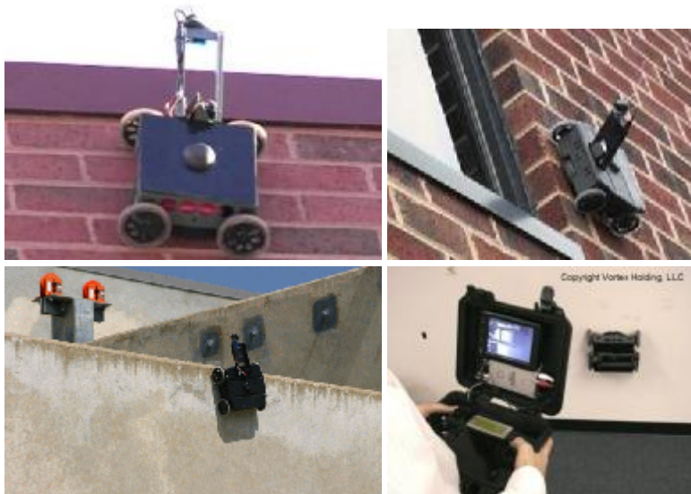
Vortex VRAM (Vortex Regenerative Air Movement) Mobile Robot Platform – motion over arbitrarily orientated surfaces
